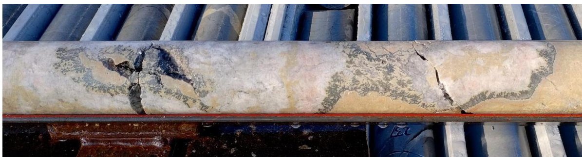
Figure 3: Drill core from BPD09 (about 223.5m down-hole depth) showing siderite (cream) and barite (white) veining. Abundant grey tetrahedrite is rimming colloform siderite-barite veining.
