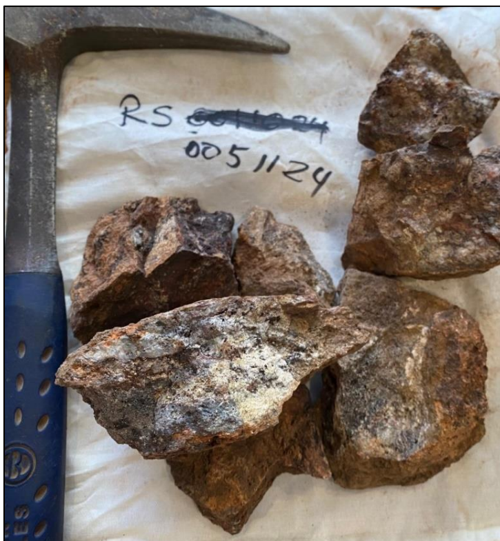
Figure 6. Sample R0051124 from Appaloosa showing iron oxide stained quartz veins in gabbro
