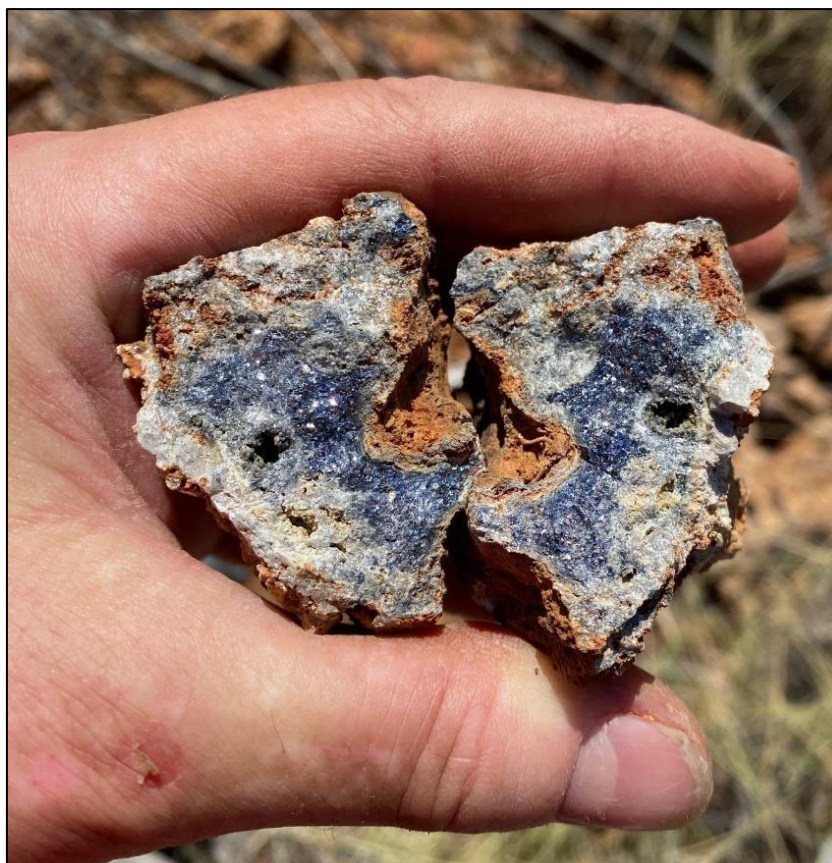
Figure 5. Sample RS0061024 from the Pickand's Showing displaying massive galena and iron oxide staining in silicified mafic volcanic.
