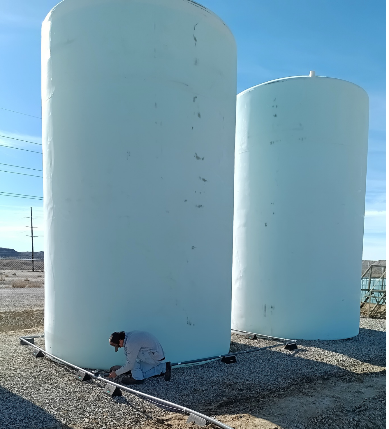
Figure 4: Two full tanks containing 32,000 gallons of lithium eluate processed by the Koch DLE at Green River, Utah, USA
