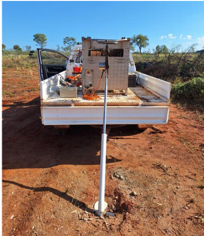
Figure 3: Jimmy Woodser Project – Downhole electro-magnetic survey at drillhole JWRC0012.
