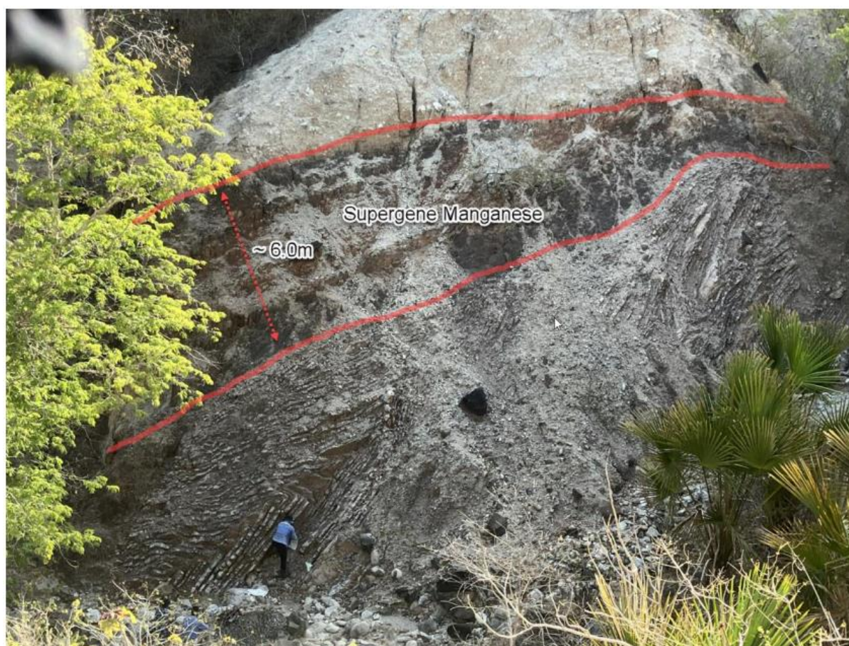
Figure 2: Estrella Geologist Kharol Varela mapping and sampling chert bedding below supergene development in an exposed outcrop. The scree from this exposure exhibited >70% manganese-iron-oxide minerals.
