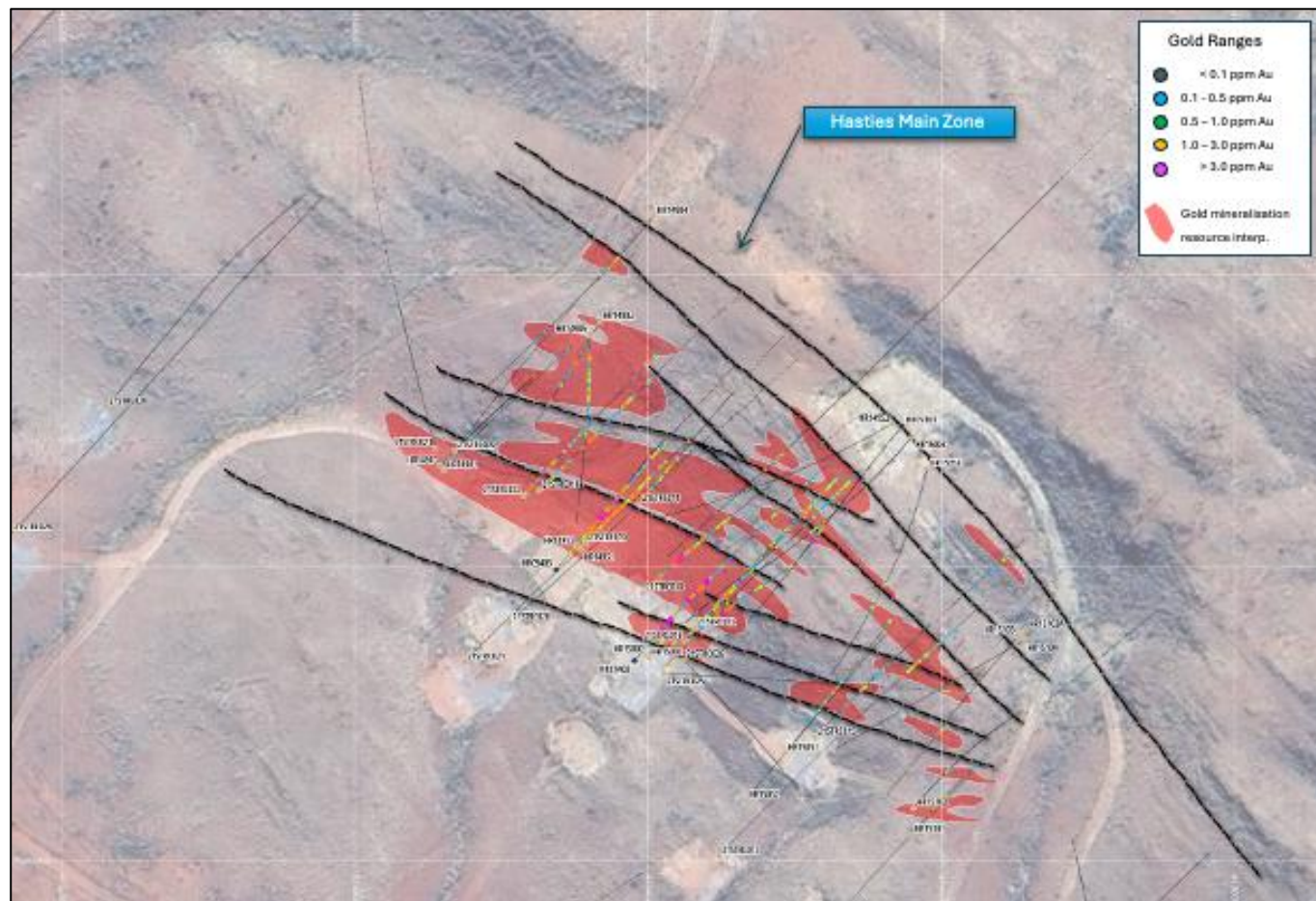
Figure 7 – Map of Hasties Main Zone deposit mineralisation model used for the estimation of a mineral resource.
