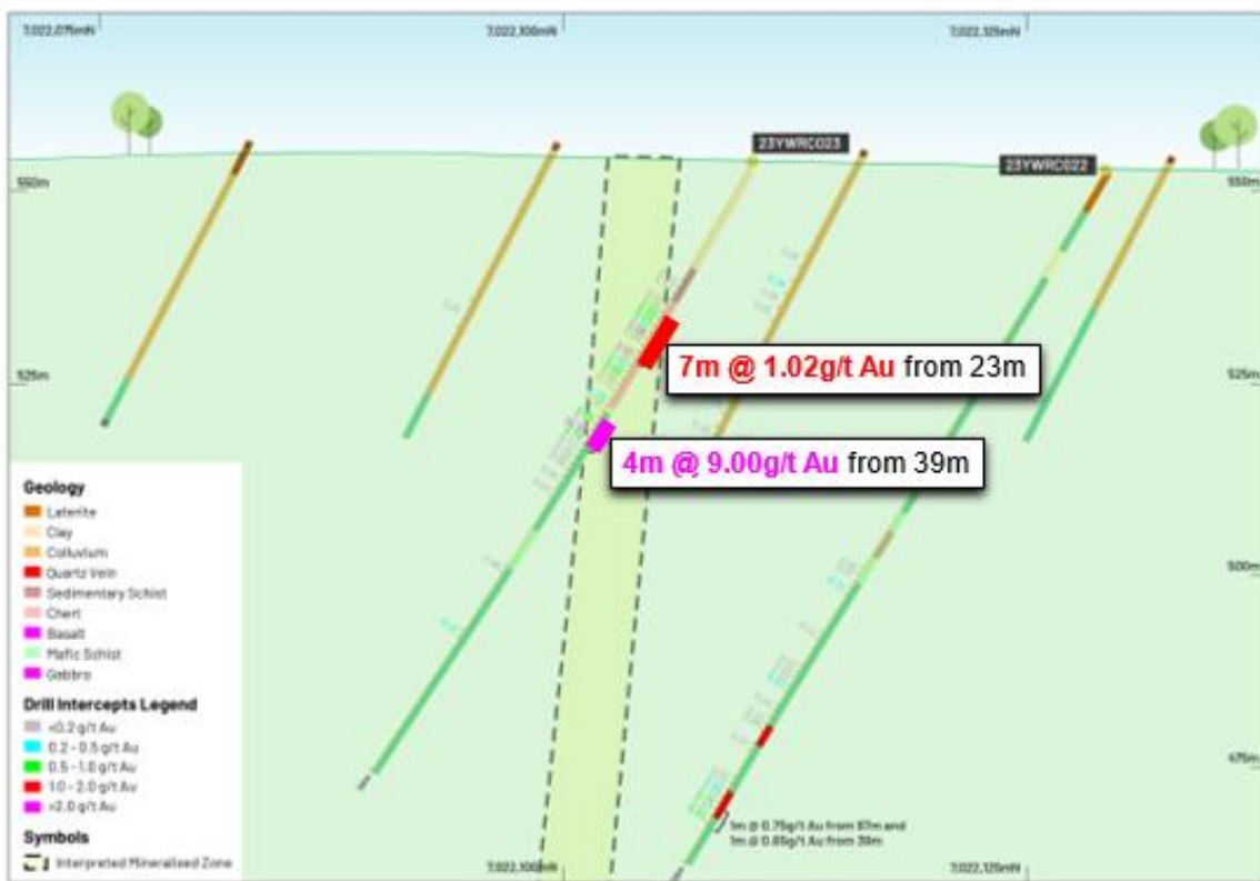
Figure 2: Cross section at Barwidgee Fault Prospect drilling.
