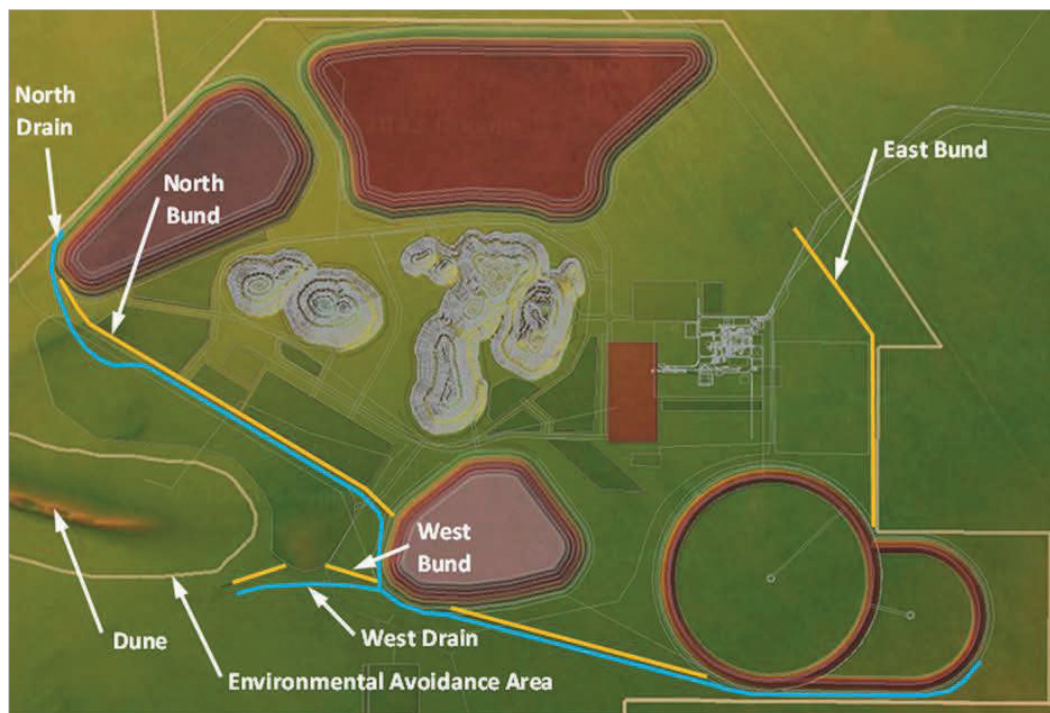
Figure 4.2 Bunds and drains incorporated into hydraulic model
