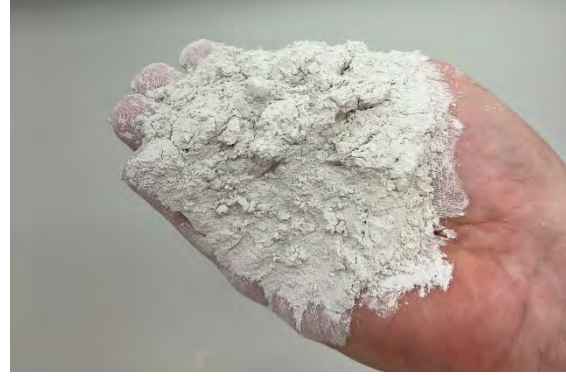
(left) four pallets of milled Toondoon kaolin ready for calcination and production of AusPozz™ HRM (right) AusPozz™ HRM produced from one of the calcination test batches
