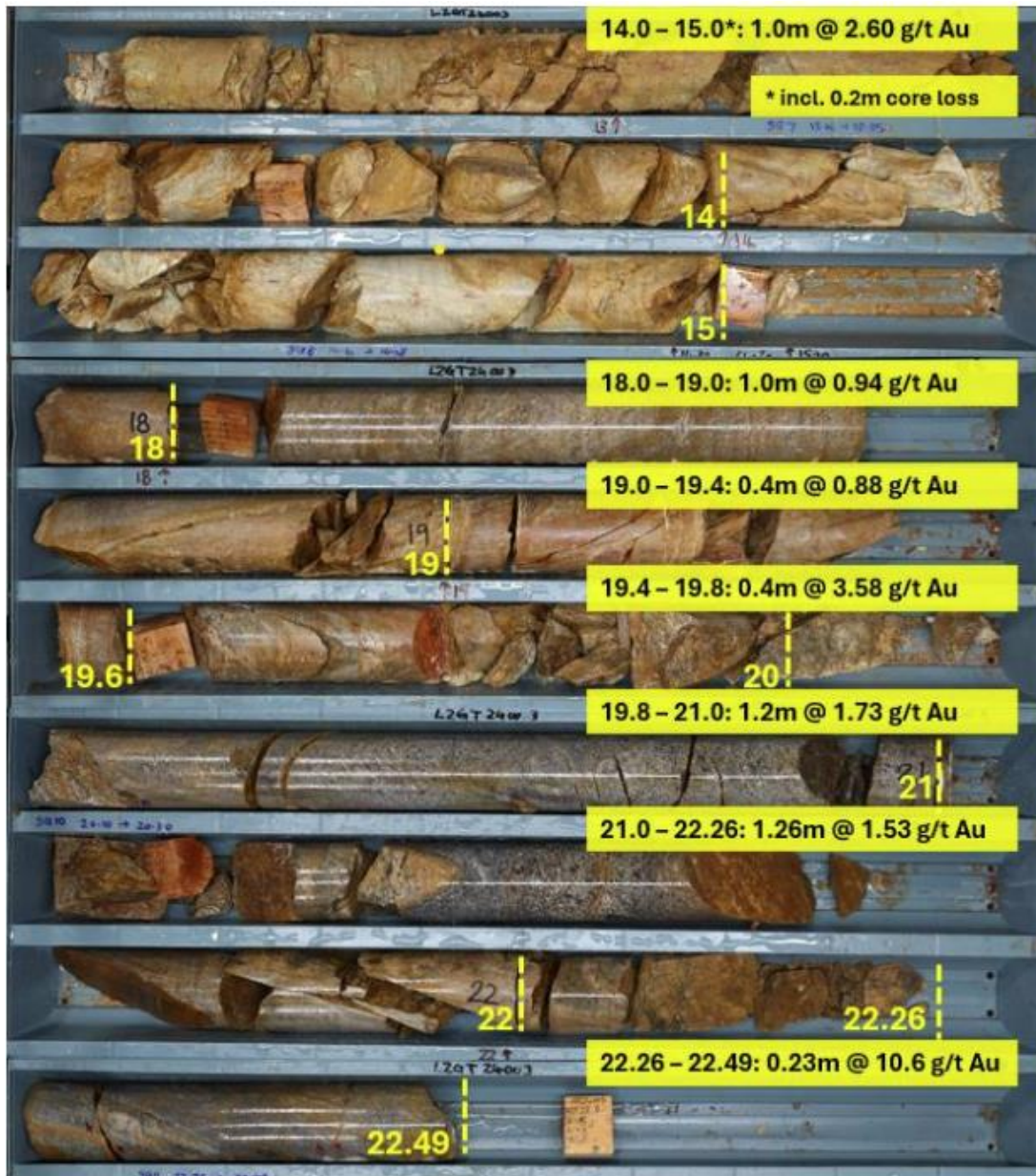
Figure 6: LZGT24003 displaying typical Link Zone oxide/transitional mineralised zones within broader 8.49m @ 1.56g/t (from 14m) intercept at Merriyulah
