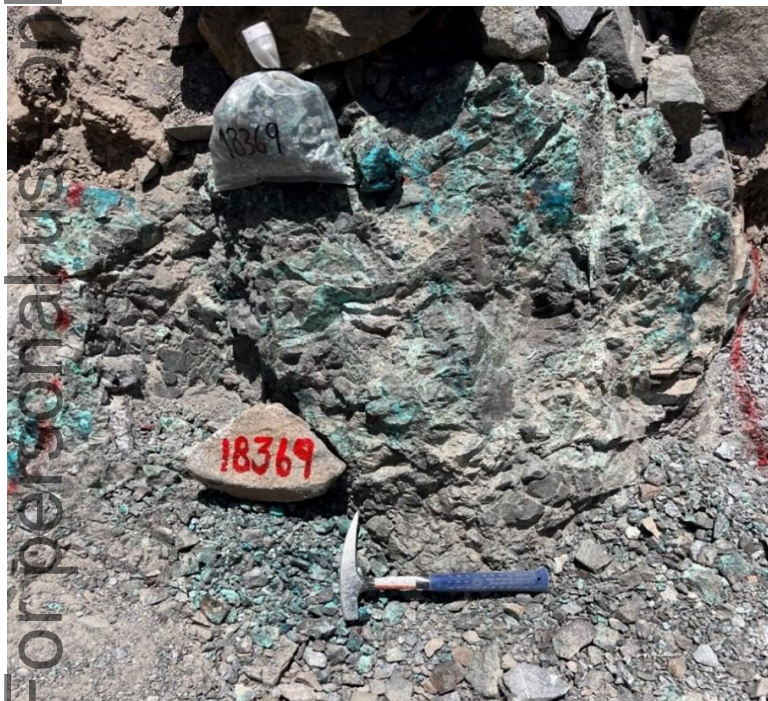
Cinto Project Channel 7, sample 18369, taken across mineralisation in brecciated andesitic tuff exposed by gully erosion. Sample length 1.1m. Assay results: Au 0.535 g/t, Ag 25 g/t, Cu 8.7%, Mo 1 ppm, Pb 283 ppm, Zn 873 ppm.
