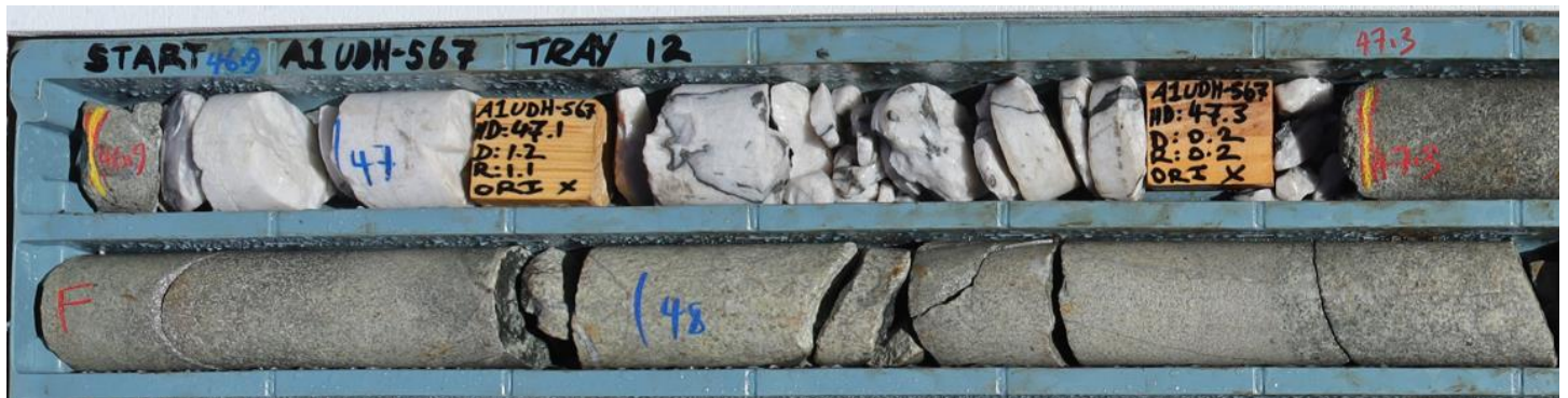
Figure 2: Drillhole A1UDH-567 showing the second mineralised intercept
