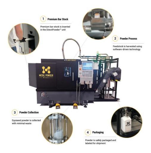
Features such as the size, shape, and distribution of particles can be controlled to create extremely consistent powder feedstocks.
