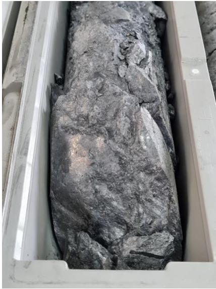
Figure 3: Photos of graphite from the Burke Deposit recovered from core drilling in January 2023 13
