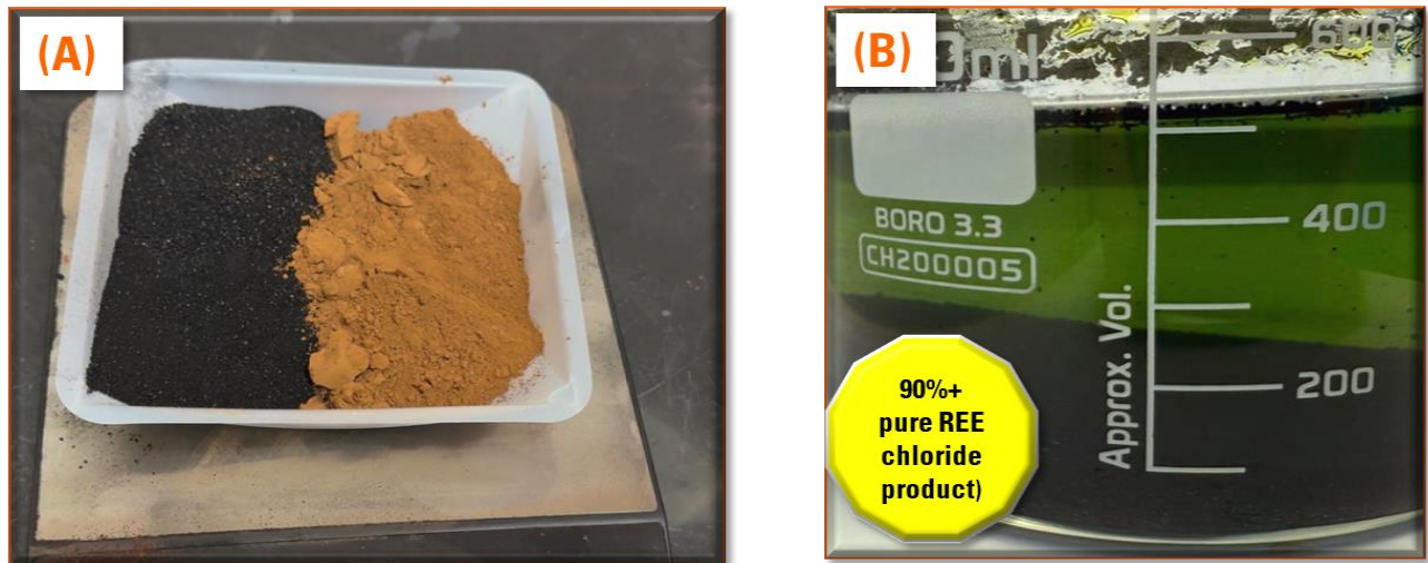
Figure 4: Photos of (A) Pre-Flash Sample of Feedstock (Flotation Concentrate) (RHS) with carbon (LHS), & (B) High purity REE-chloride product (>90% purity) produced from water-washing the post flashed solids
