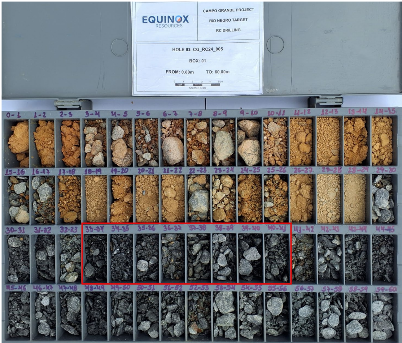
Figure 2: Rock chip tray from Hole CG_RC24_005 at the Rio Negro Target, displaying samples from 0m to 60m depth. The interval from 33–41m highlights the transition from reddish-brown, friable material associated with supergene alteration to darker, compact lithology indicative of primary monazite-bearing mineralisation.
