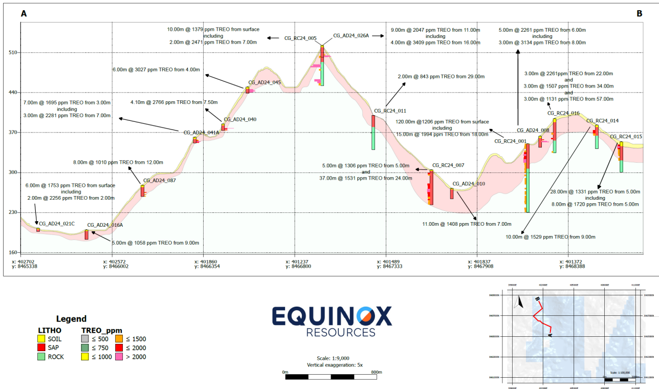
Figure 3: South to North 2-D Fence diagram of the Rio Negro Target, illustrating mineralised intervals across multiple RC drill holes. Key intercepts highlight high-grade TREO zones, including 5m at 6585 ppm TREO (Hole CG_RC24_005). The diagram also showcases the lithological distribution of soil, saprolite, and rock, with TREO concentrations exceeding 2,000 ppm in several intervals, reinforcing the target's rare earth mineralisation.
