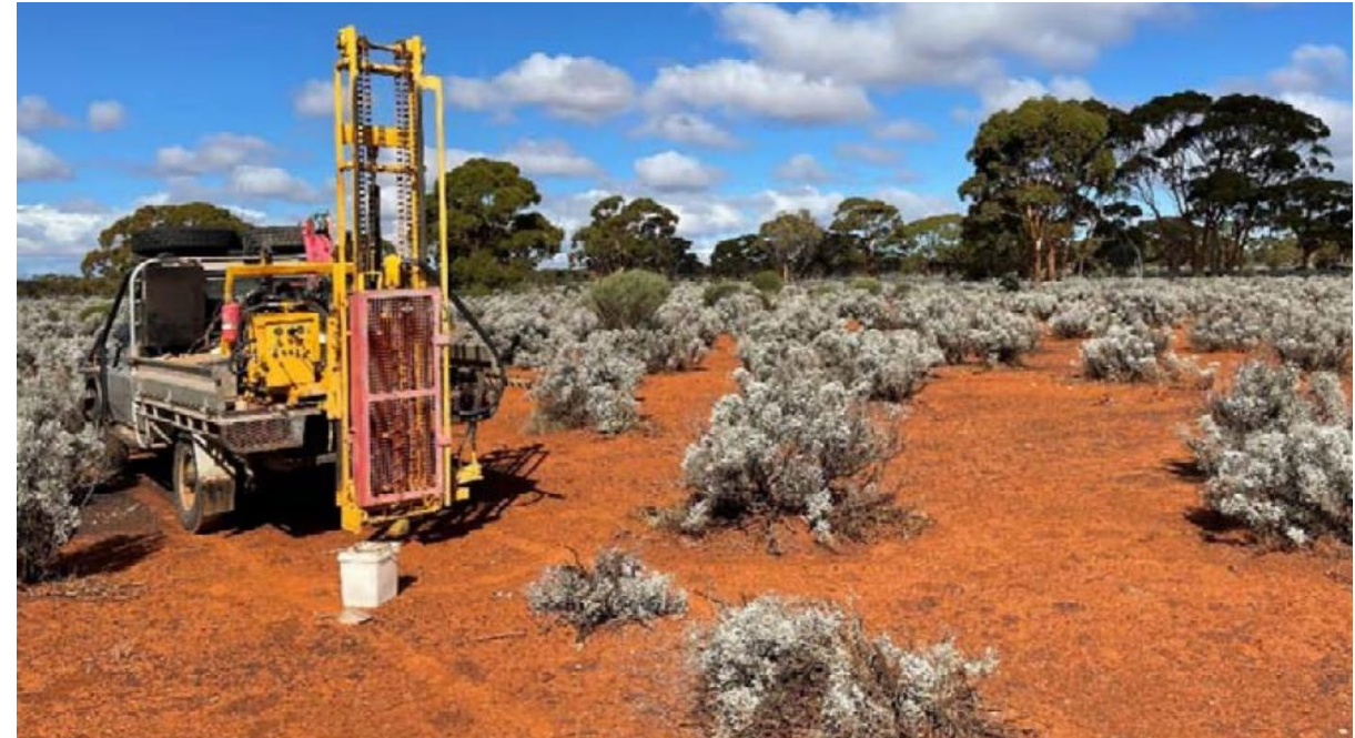
Auger rig used for calcrete sampling
