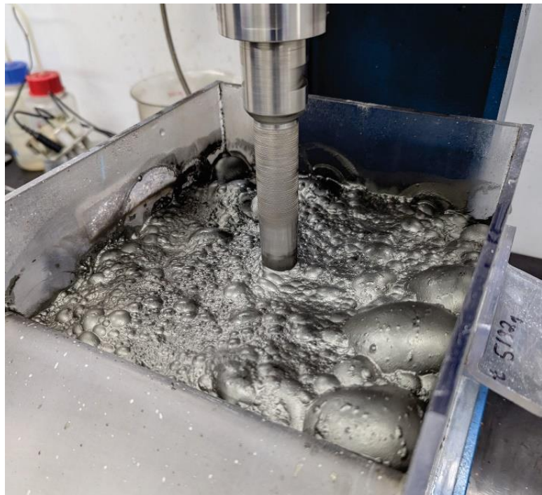
Figure 1: Copper-antimony concentrate from Bulla Park, first floatation test run, at Core Resources laboratory
