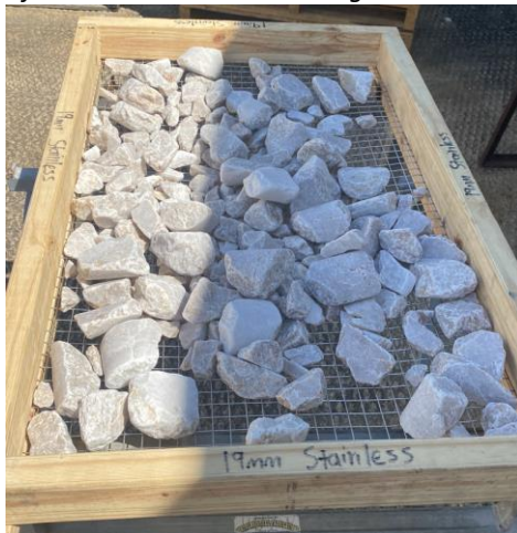
Figure 1 – Crushed, screened and scrubbed +19mm – 100mm quartz lump from Quartz Hill prepared for Sensor Based Ore Sorting Trials at TOMRA in Germany
