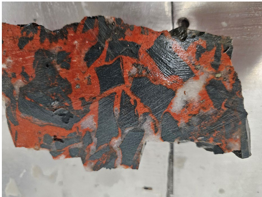
Figure 5: Brecciated host shale with infill of quartz and intense potassic feldspar alteration (orange-red) and sulphide aggregations
