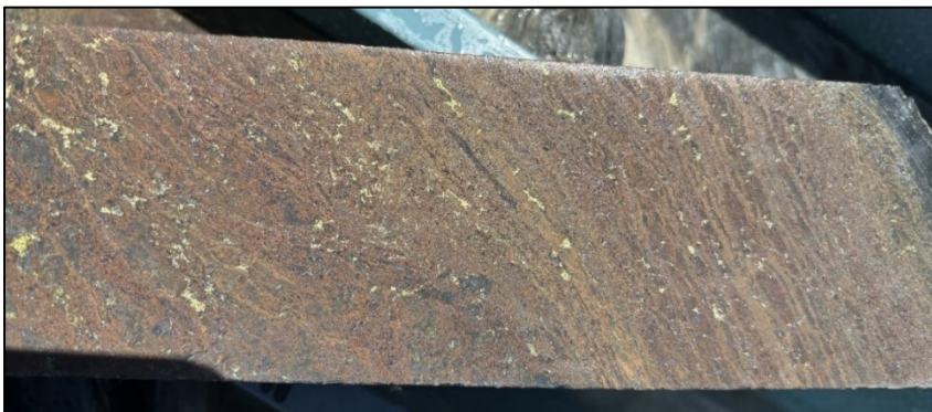
Figure 1: ~20cm zone of high-grade drill core from A3DD007 from within interval 140.1-140.9m, which graded 4.5g/t Au, 2,010g/t Ag, 1.3% Cu & 16.1% Pb+Zn.
