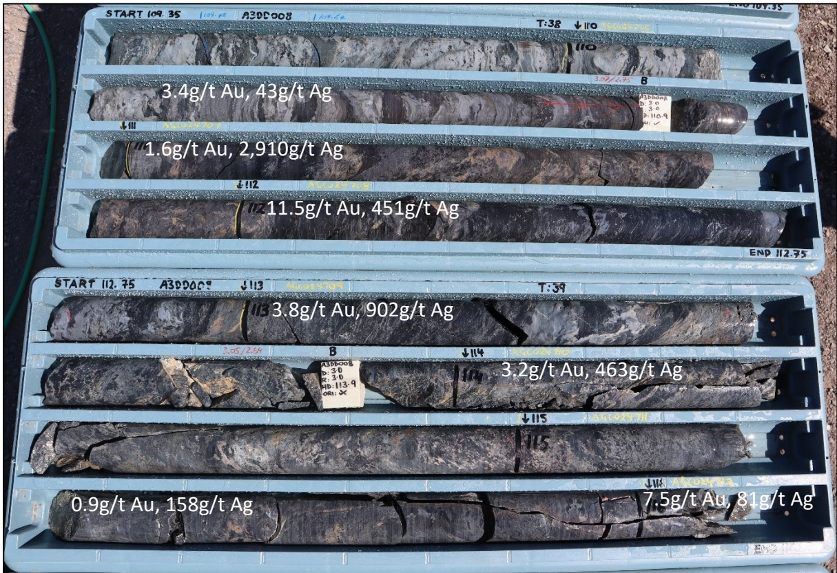
Figure 3: Core photographs of most of the 9m wide, high grade silver-gold zone in A3DD008 grading 3.7g/t Au, 566g/t Ag & 1.4% Pb+Zn from 110m.
