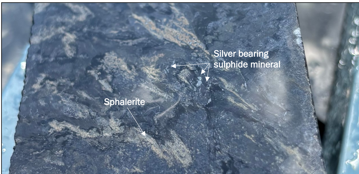
Figure 4: Core photographs of silver coloured dendritic minerals of the silver bearing sulphide mineral tennantite within A3DD008 high silver interval 111-112m with 2,910g/t Ag.
