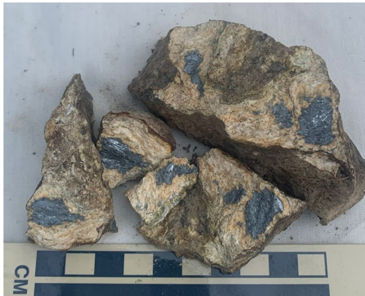
Sample MVS14: 31.8% Antimony and 0.84grams/tonne Gold. Silicified, grey pelite hosting a 30mm wide vein of white and minor pale green antimony oxide (antimony trioxide Sb_2O_3 ), and portions with silvery-grey antimony sulphide (stibnite, Sb_2S_3 ). Clumps of stibnite up to 20mmx12mm. Also 2mm wide quartz veins with Fe-Ox (scale bar: Centimetre divisions).
