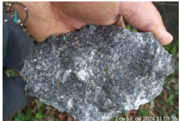
Figure 7: Coarse-grained nepheline syenite with a coarse equi-granular texture formed by the intergrowth of feldspar, nepheline, and mafic minerals
