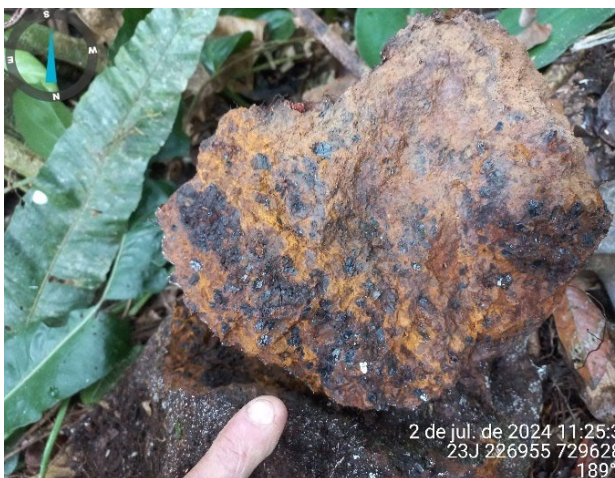
Figure 8: Segregated magnetite-rich layers alternating with heavily altered ferromagnesian minerals, likely of olivine origin (JUQ-RO-0022)
