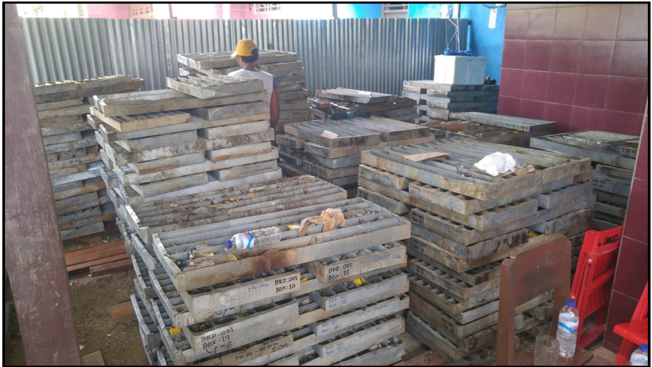
Photo 5 : Coreboxes from Bermol, Mafi, Sikrima and Silia prospects neatly stacked in an undercover garage at the Arso storage facility. Note the coreboxes are cross-stacked to lessen the possibility of toppling over in the frequent earthquakes that strike this area.
