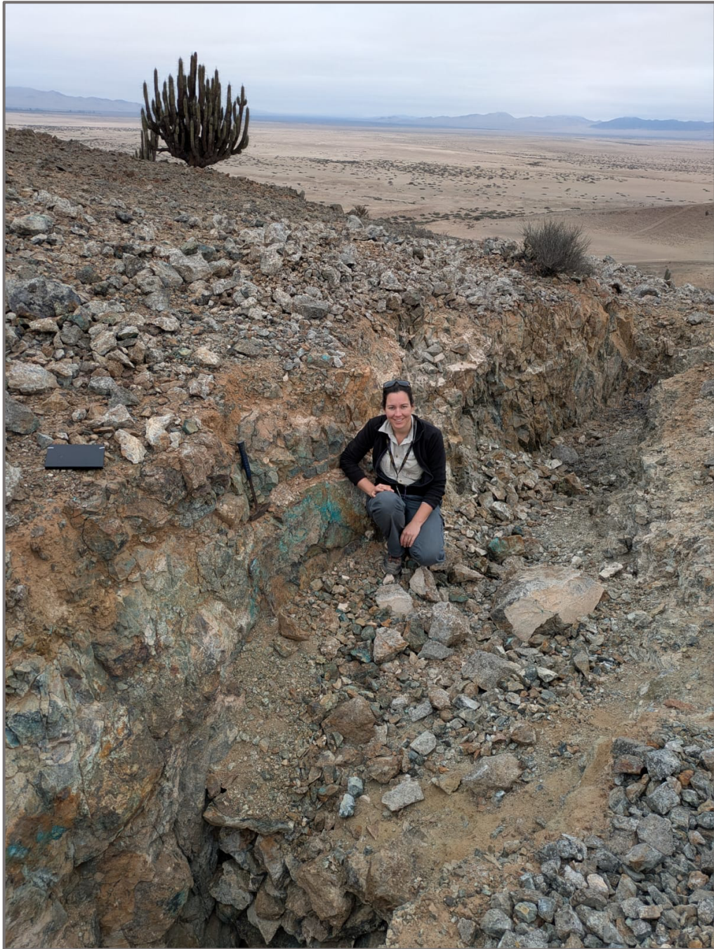
Figure 4: Historic workings within a +1km trend that has rock chip assays of 3.4% Cu and 63.4% Fe above a magnetic anomaly.
