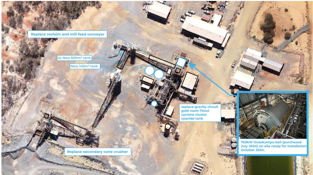
Figure 38 – Andy Well CIL process plant layout.
