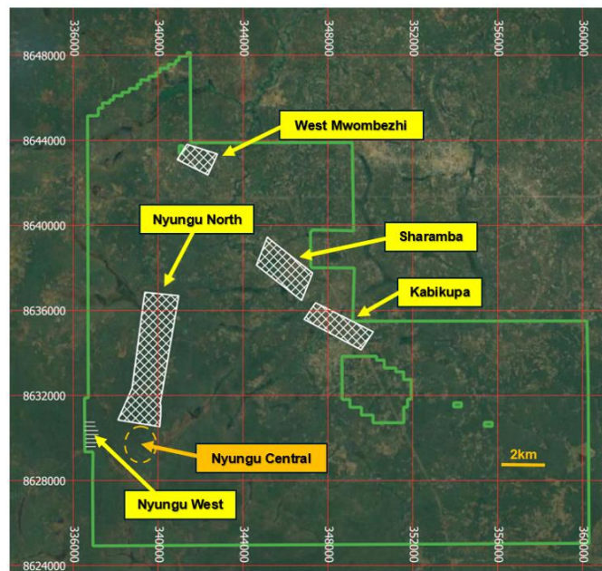
Figure 1: Mumbezhi exploration licence showing grid locations of IP surveys in relation to the Nyungu Central copper deposit (orange ellipse)
