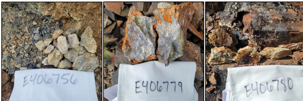
Figure 5. Samples E406756 (17.6 g/t Au, 0.1% Sb), E406779 (18.1 g/t Au, 0.6% Sb) and E406780 (62.3 g/t Au)
