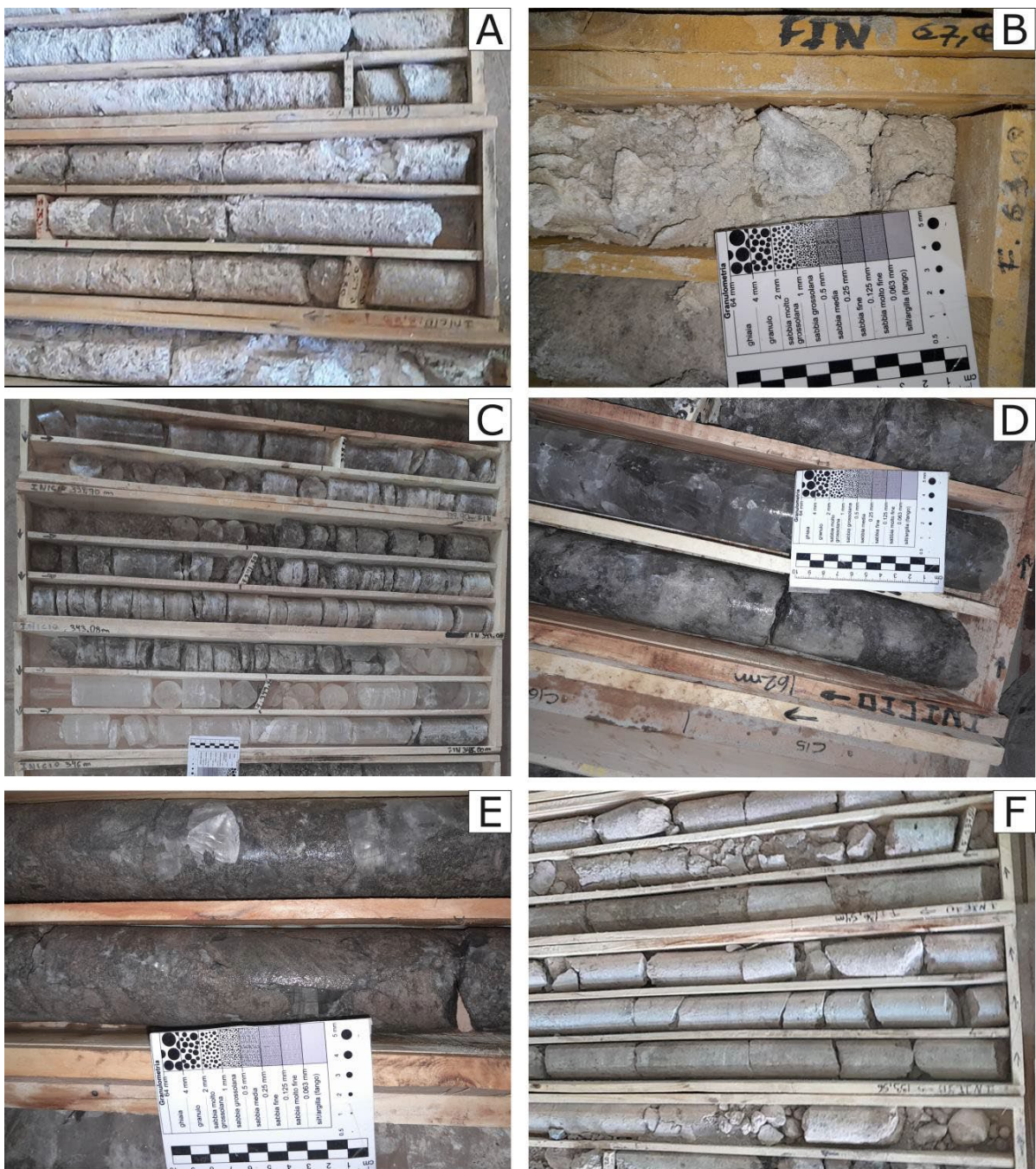
Figure 5 – Main lithologies as described in hole DDH-1. A: Sulphates B: Sand with gypsum. C: Discoidal Halite. D: Halite with matrix. E: Sand with gypsum. F: Sand
