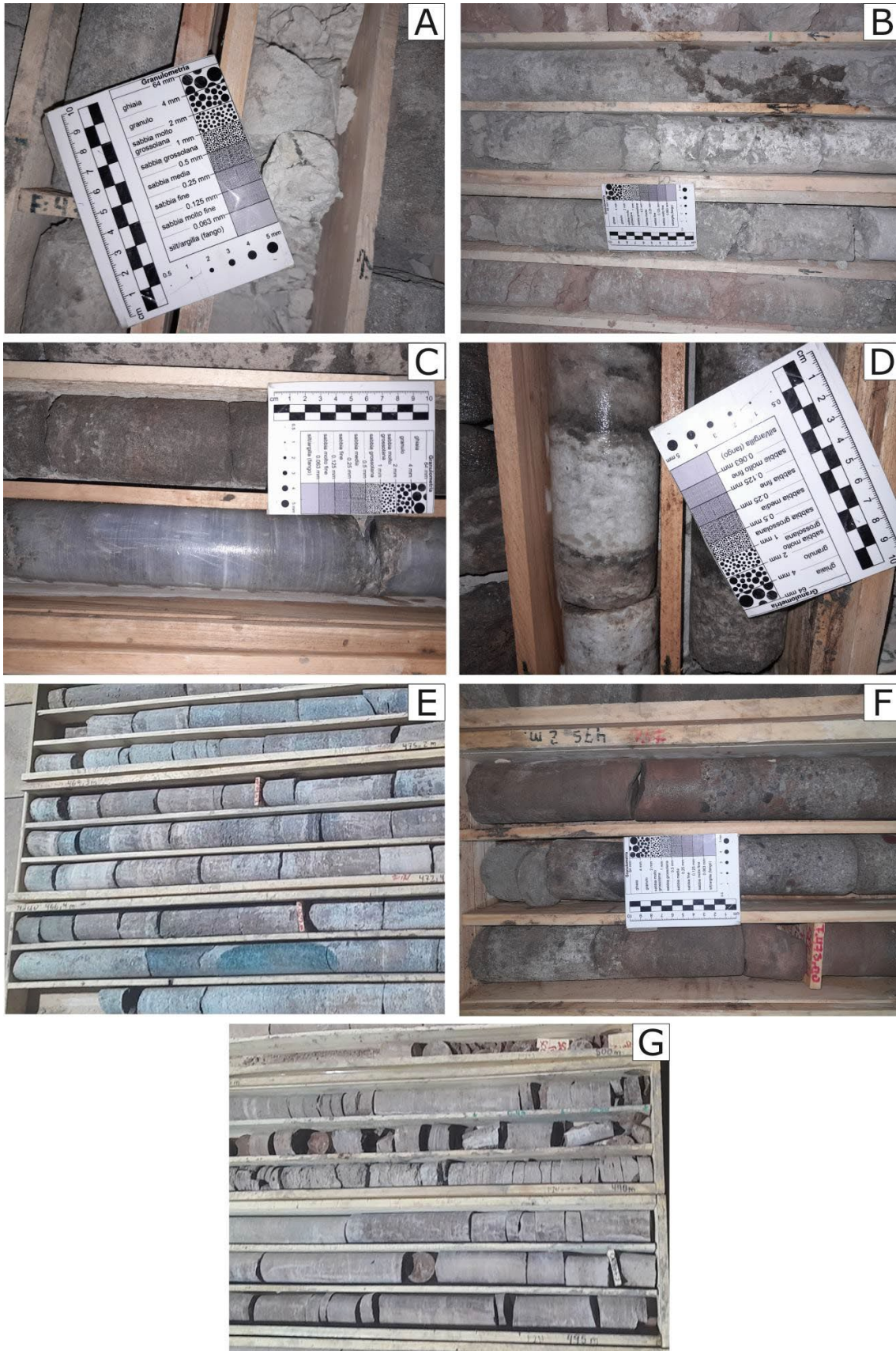
Figure 6 – Main lithologies Main lithologies as described in hole DDH-2. A: Gypsum B: Sand with gypsum. C: Anhydrite. D: Anhydrite with sand. E: Sand. F: Gravel. G: Sand with clay.
