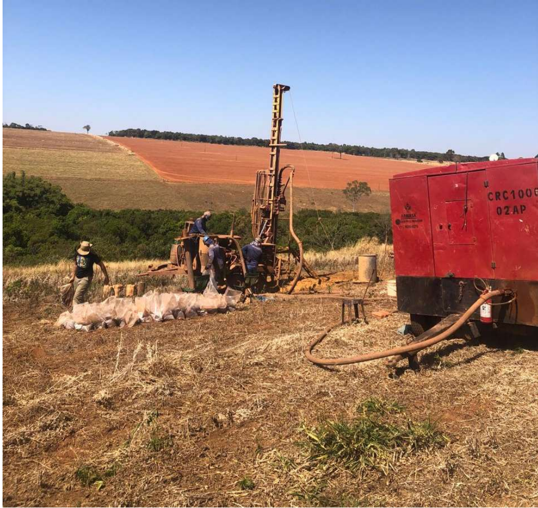
Figure 1: RC drilling rig in CODA North Project site operating in our REE mineralisation area (Sample bags are arranged in an array prior to logging and transferring to sample shed)
