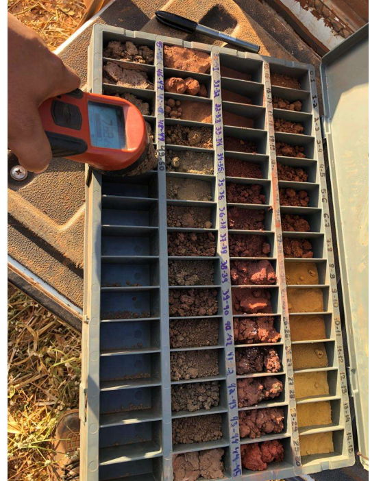
Figure 7: Enova's professional geologist is checking the magnetic susceptibility of saprolite drill cuttings during logging
