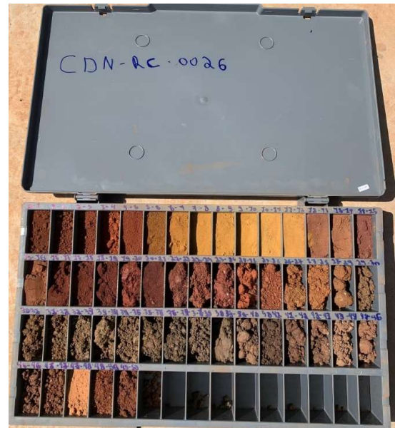
Figure 9: Variegated colour of drill cuttings implying changes in lithology across undifferentiated sediment, laterite, kamafugite
