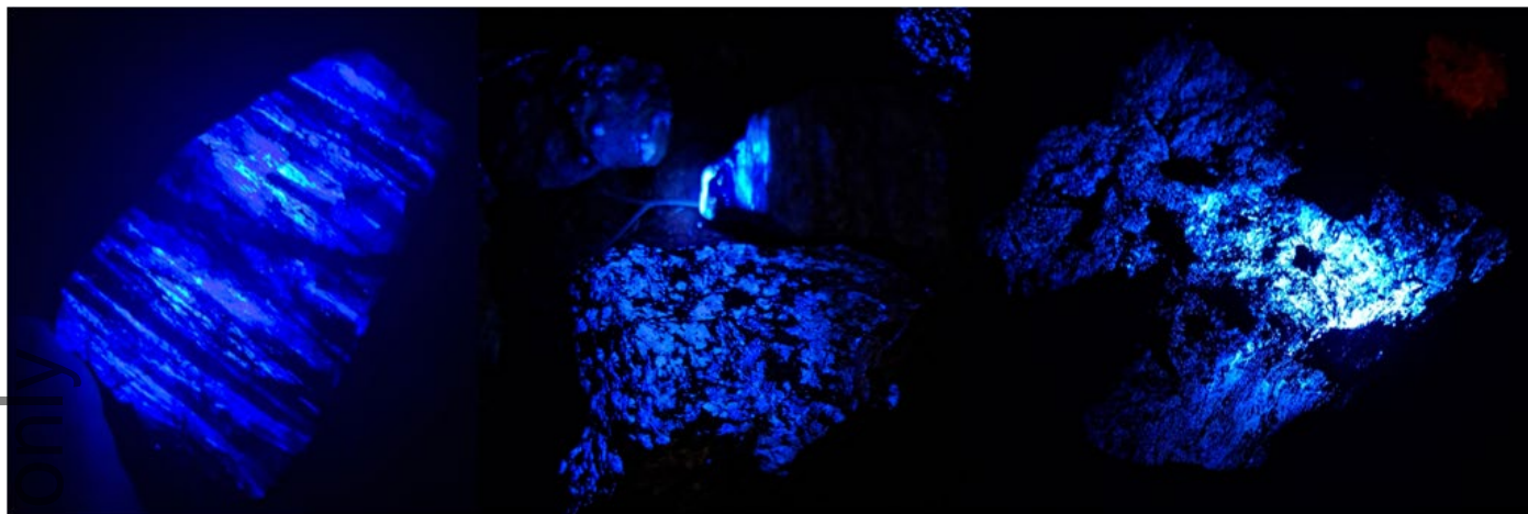
Figure 5 – Examples of scheelite bearing samples identified by UV light in containment bunds and on waste rock dumps at Western Queen. Note: samples shown are not to scale.
