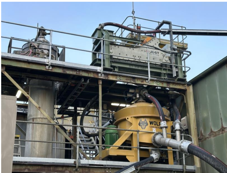
Figure 3: Wolff Batch Centrifugal Concentrator – coarse gold gravity collector
