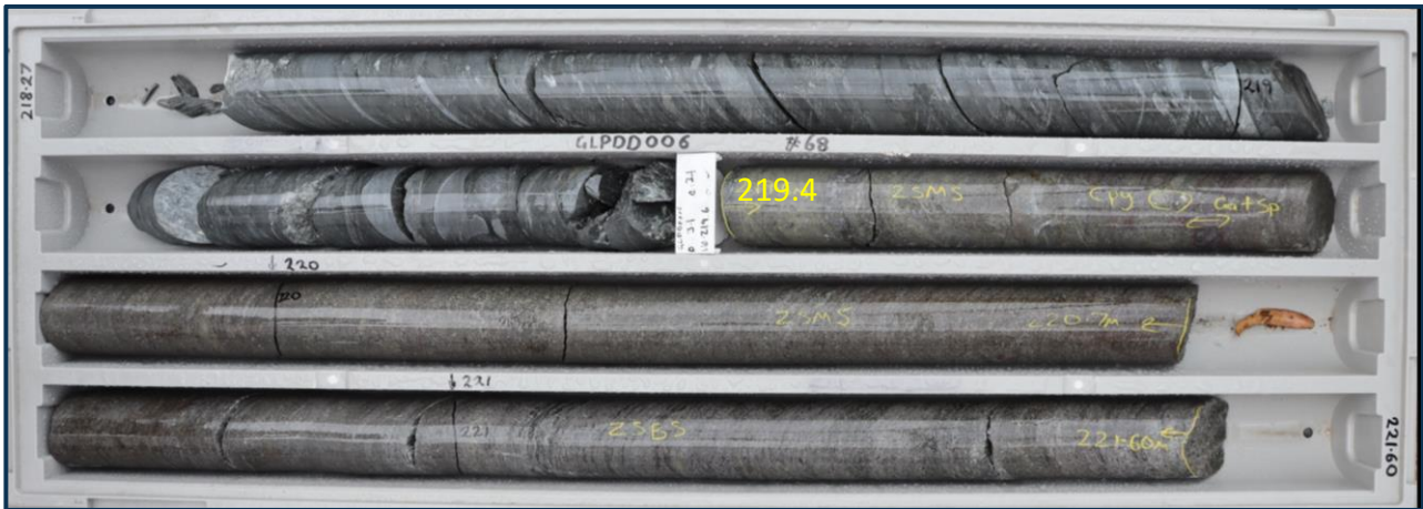
Figure 4: Diamond drill core interval 218.27-221.6m from the Spicer's Lode in GLPDD006. Summary geology: 218.27 – 219.4m: mixed provenance breccia; 219.4 - 220.7m: massive to semi-massive sulphide with - in order of abundance - pyrite, sphalerite, galena (refer Appendix 1).
