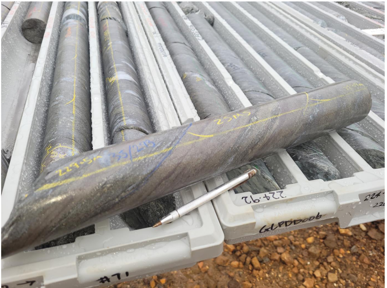
Figure 2: Photo of diamond drill core from GLPDD006 showing massive to semi-massive sulphide lode showing banded pyrite (yellow) and sphalerite (red) with galena and chalcopyrite (refer Appendix 1)
