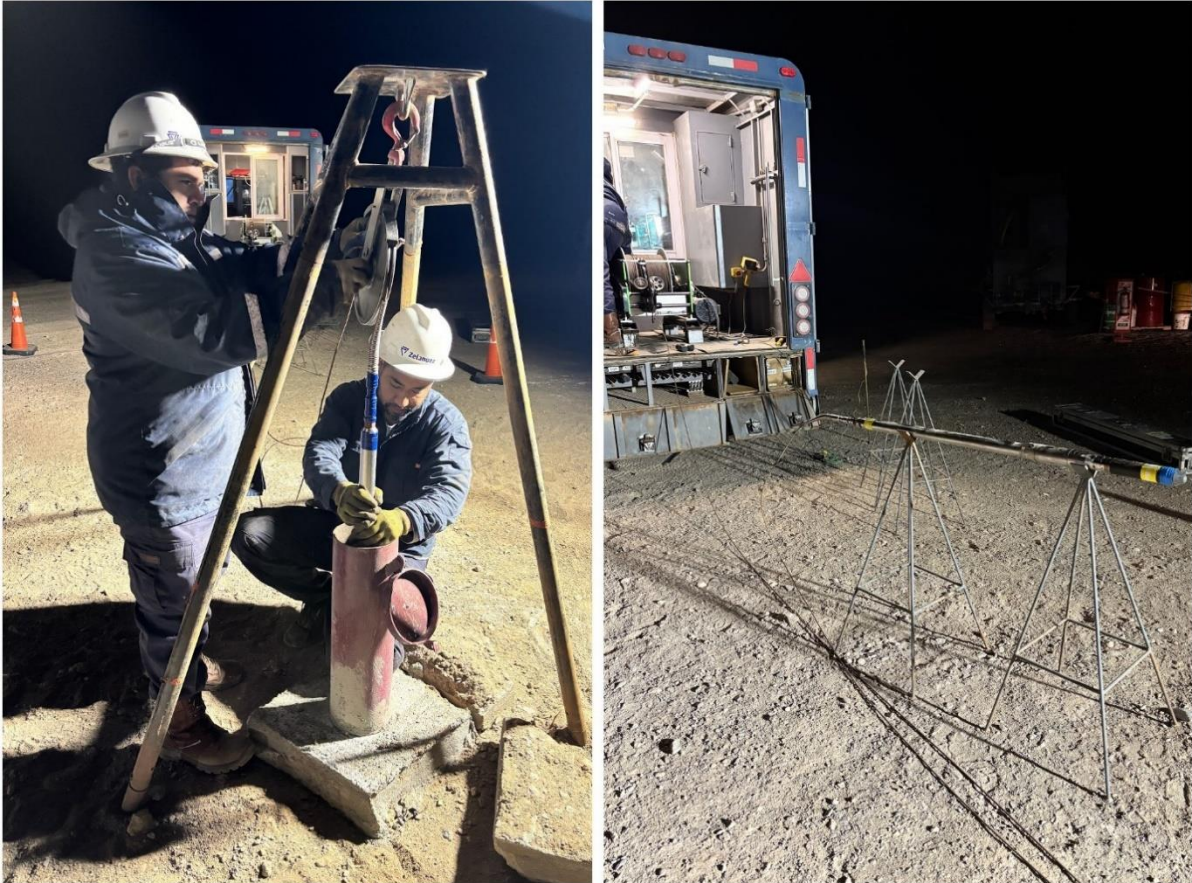
Figure 1. Geophysicists setting up the nuclear magnetic resonance tool to take gamma, conductivity and resistivity readings.
