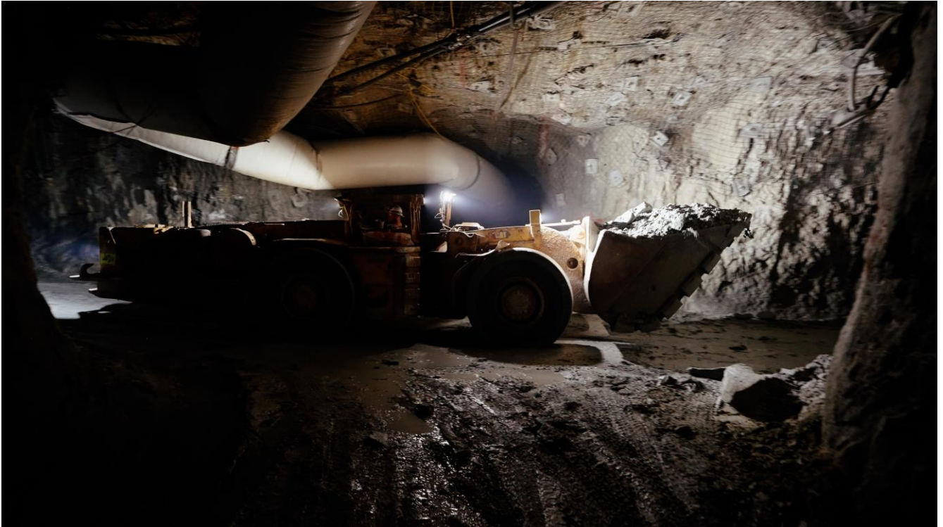
Figure 6 - CAT 1700 loader bogging an ore stockpile to a waiting truck on the Decline
