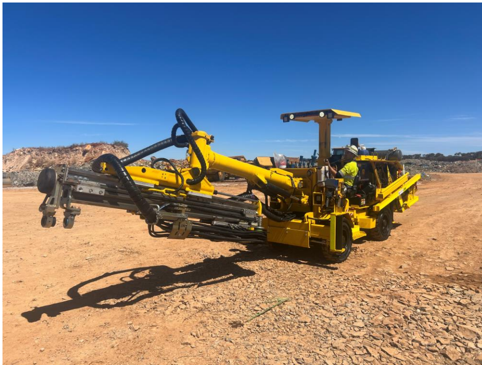
Figure 1 – Zero hour rebuild Atlas H104 development drill arriving at Second Fortune
