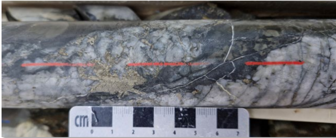
Figure 4: CUTBD03, 145m – Unsampled pyrite(brass-yellow)-pyrrhotite (brown-bronze) in quartz vein (see Appendix 1, Drill Log Summaries and Cautionary Note Page 2).
