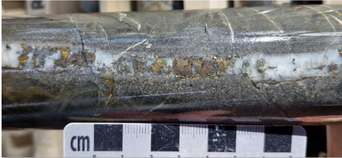
Figure 10: CUTAD01, 225.3m - Unsamplered pyrrhotite (brown-bronze)-chalcopyrite (yellow)-pyrite (brass yellow) in quartz vein (see Appendix 1, Drill Log Summaries and Figure 3 Cautionary Note Page 2).
