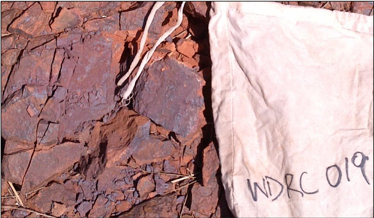
Figure 5. Sample WDRC019 - 64.3% Fe. Refer to Figure 3 for the photo and sample location
