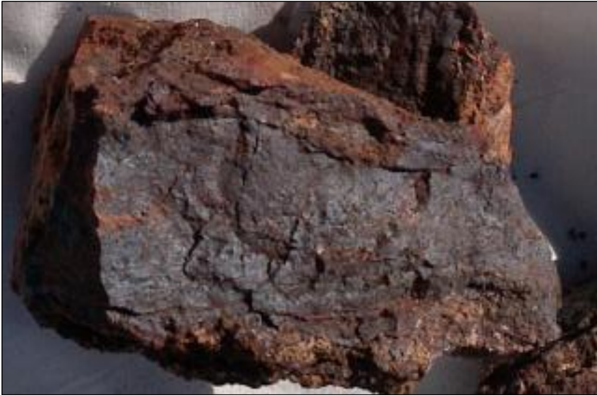
Figure 7. Sample WDRC005 - 63.3% Fe 1 . Refer to Figure 3 for the photo and sample location
