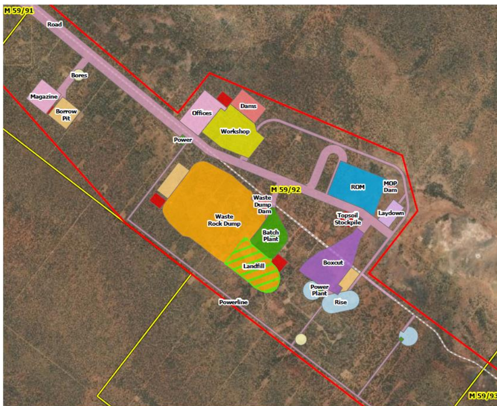
Figure 13: Site layout and infrastructure
