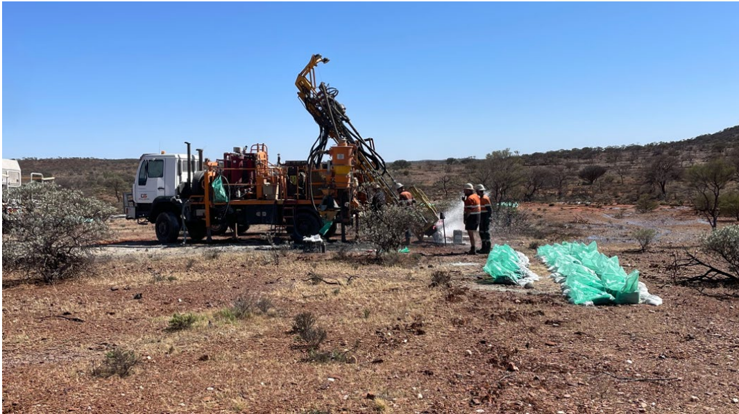
Figure 2 RC rig in action at the Austin Gold Project
