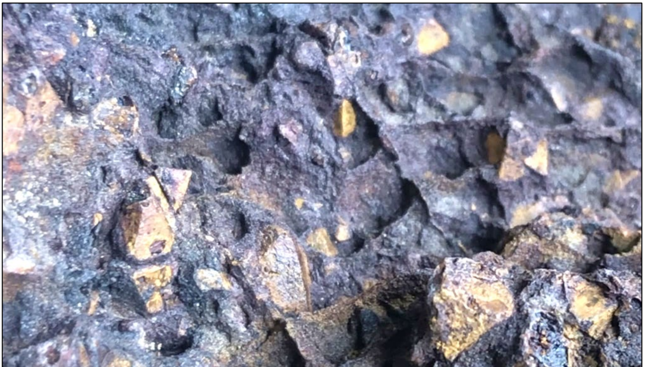
Figure 1: Remnant chalcopyrite crystals in heavily boxworked gossan sample (rock chip returned 0.59% Cu, CO24_008, 1kg sample). Photo field of view ~1cm x1.5cm.
