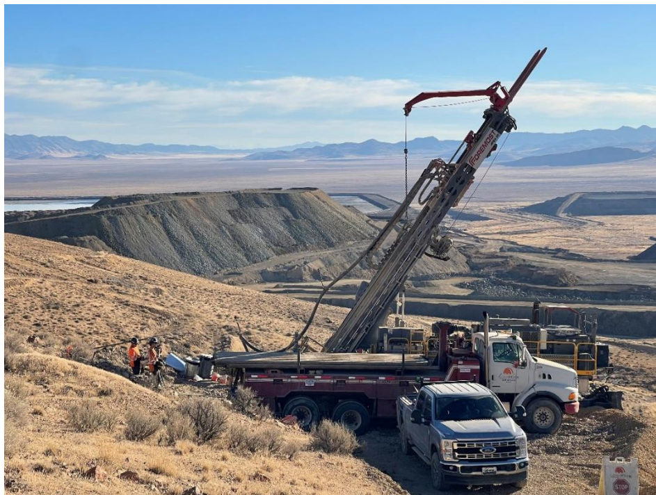
Figure 3: Reverse circulation (RC) drill rig set up ready for drilling at the Independence Gold Project.
