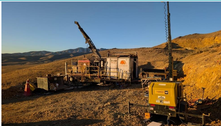
Figure 2: Diamond drill rig setting up at the first drill site at the Independence Gold Project.
