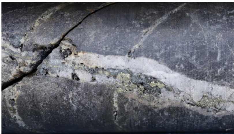
Figure 2 Strongly mineralised volcaniclastic sediments at 35.9m depth in hole 24BRD0031. Sample assayed 1.16% Cu and 55ppm Mo. Note multiple quartz-chalcopyrite-pyrite-chlorite veining events. Core diameter 61.1mm
