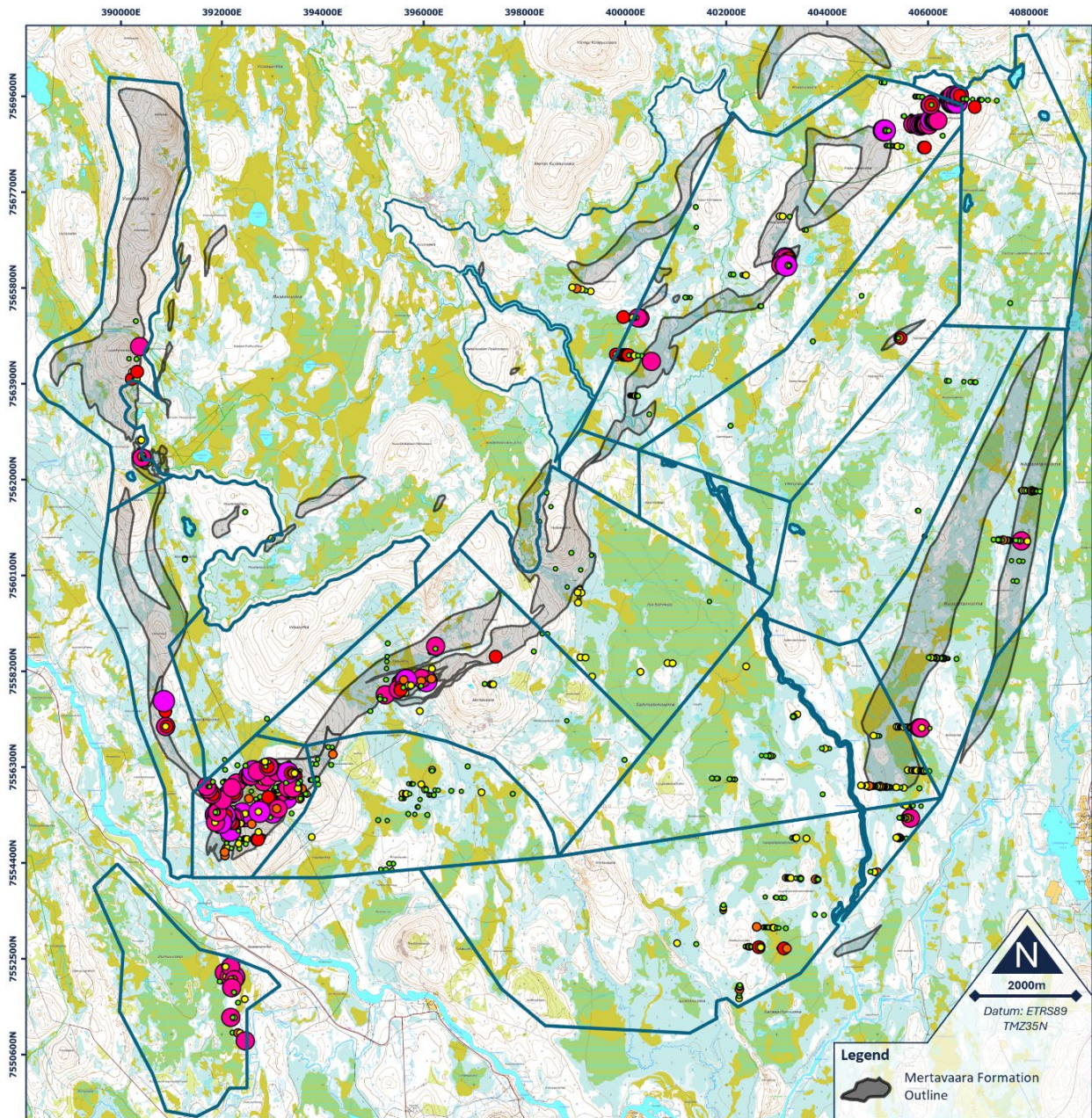
Figure 2: Nickel anomalism as mapped by BOT drill samples. The grade and percentile ranges are as follows: Blue: 374-464ppm (88-90 th percentile); Green: 468-920ppm Ni (90-94 th percentile); Yellow: 931-1507ppm Ni (94-96 th percentile); Orange: 1517-1862ppm Ni (96-97 th percentile); Red: 1880-2400ppm Ni (97-98 th percentile); Magenta: 2413-3765ppm Ni (98-99.6 th percentile); Pink: 3838-17710ppm Ni (99.6 th percentile and over). (Source: OKU detailed till geochemistry, modified data © Geological Survey of Finland 2024)
