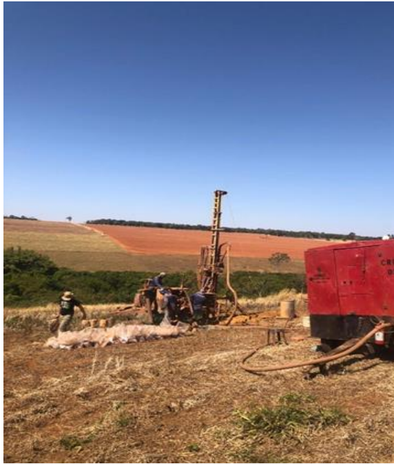
Figure 6: Reverse circulation drill rig in the backdrop of vast pastureland of CODA North. Plastic sample bags are arranged prior to transfer to the sample shed
