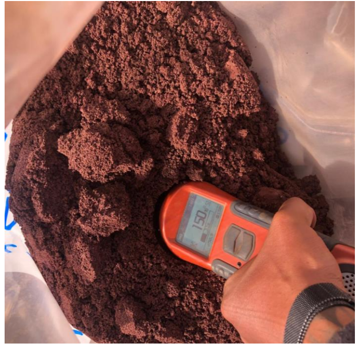
Figure 7: Enova's professional geologist is checking the magnetic susceptibility of saprolite drill cuttings during logging
