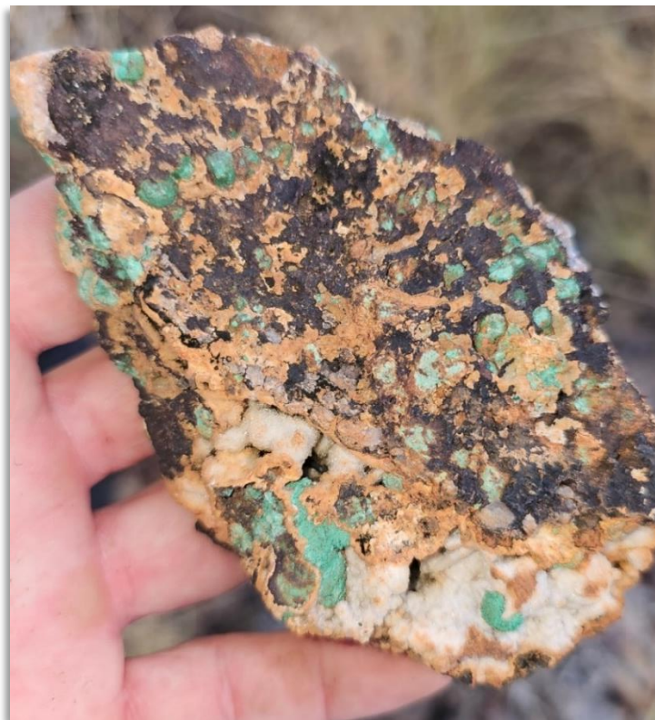
Figure 4 - Vuggy quartz breccia with abundant malachite. Sample from the Peter prospect, Mt Isa (304,045mE 7,908,330mN GDA2020 z54). Assays of 20.9% Cu and 8.54 g/t Ag (AR28612). Field of view is 8cm.
