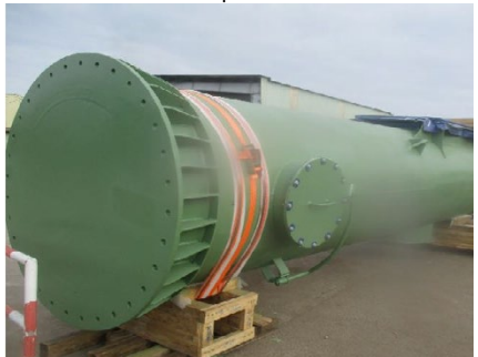
Main Venturi Scrubber
