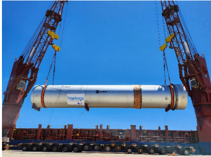
Acid Bake Kiln (weight 100 tonnes)
