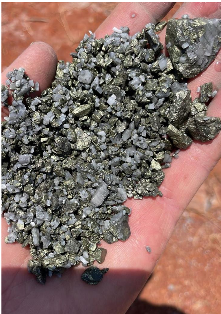
Figure 2: Copper mineralisation in drill chips during the recent Surprise prospect drill program collected from ASRC002 (44m to 45m down hole). Refer to the disclaimer above regarding visual estimates. The mineral assemblage of the interval is estimated to include 5% pyrite, 35% chalcopyrite and 60% calcite. The host rock for the mineralisation is calcite, which is hosted within a metamorphosed, magnetite and chlorite altered amphibolite.
