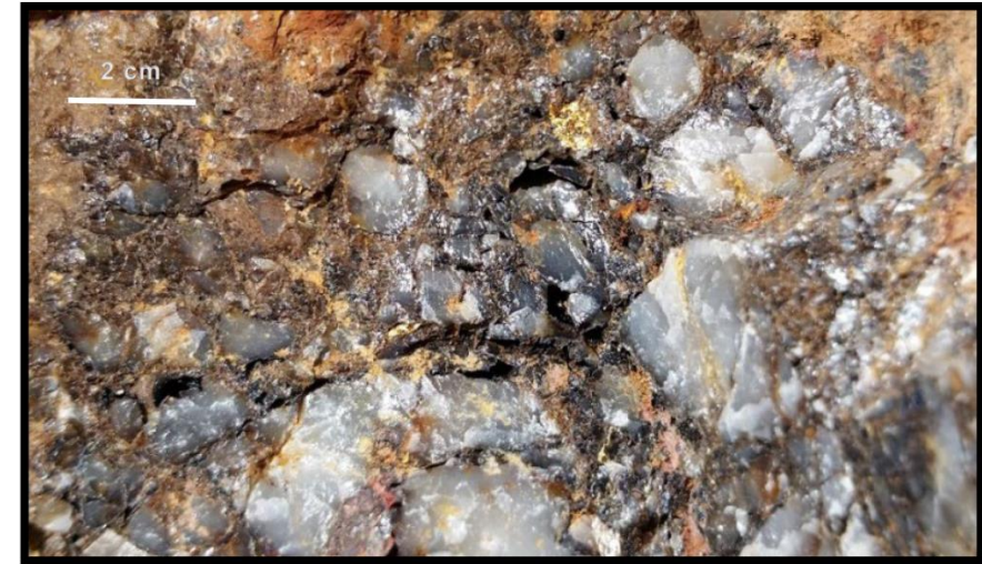
Visible gold in the Revere Reef system, about 35 cm quartz vein outcrop in shallow costean
