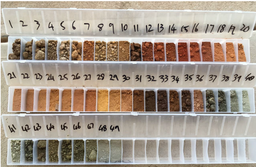
Figure 2: Chip tray for air core drill hole MA07 which intersected 18m @ 217ppm Sc from 30 metres including 6m @ 331ppm Sc from 31 metres. Numbers 1 – 49 on the chip tray denote individual downhole intervals (i.e., “10” means the drill sample obtained from 9 – 10 metres).
