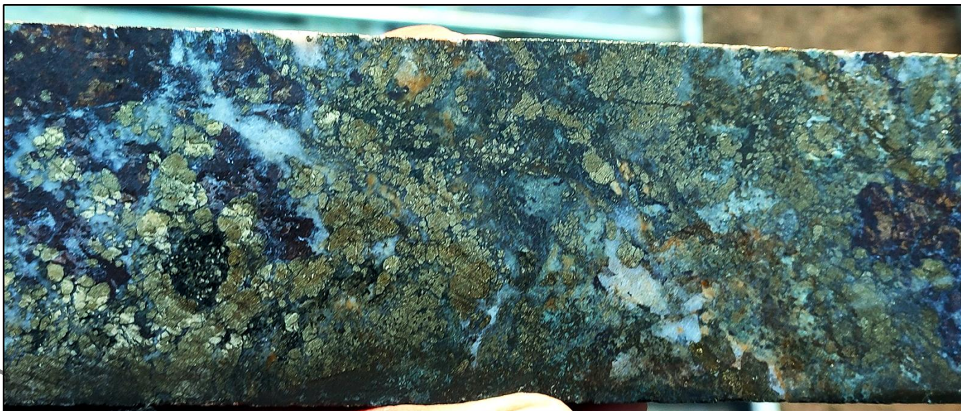
Figure 1. Core photo of high-grade polymetallic mineralisation from 354.8m in ZRSD24164 – 9.5g/t Au, 0.4% Cu, 2.1% Pb, 2.3% Zn and 60.2g/t Ag (13.1g/t AuEq).
